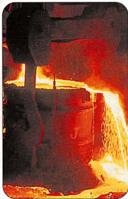
▲ Steel is a form of iron, alloyed with carbon and other metals to make it stronger. It is produced in giant furnaces.
